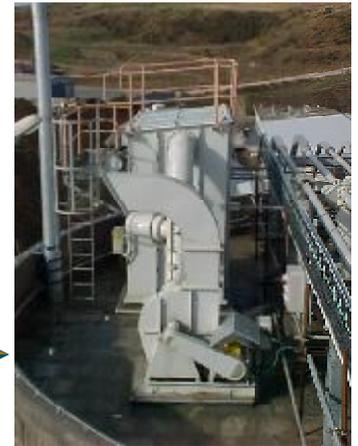
Fan Filter Unit on top of a Road Loading Bin
