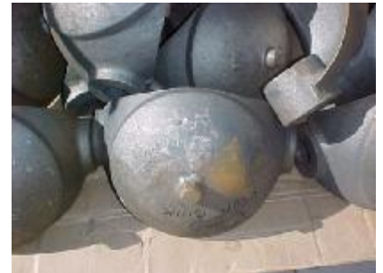
Dome Valve pressure tested and ready for dispatch ▼
