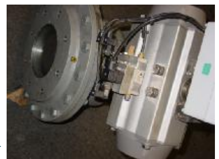
Dome Valve fitted with Actuator and PLC Control box ▼
